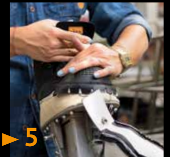
6 INSERIMENTO MEMBRANA WATER SHIELD Water Shield membrane insertion / Einsetzen Water Shield Membran
